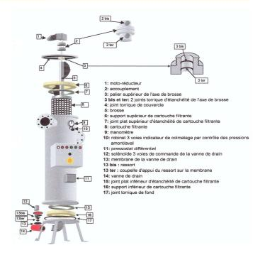
The helicoidally brush is only in the smallest model.
