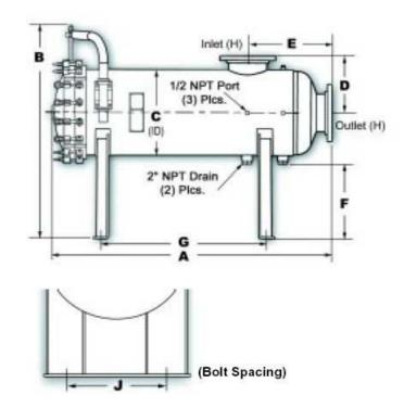
A second filtration stage with technically more sophisticated and lower cut off level cartridges. These cartridges are either wounded or folded types with performance guarantee.
